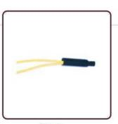
Fit Cap This is the **third step**. Place the cap over the twisted copper wire and some overlap of the insulation.
