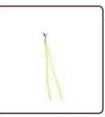
Twist Together This is the second step. Twist the pair of copper wires together almost the full length of copper.
