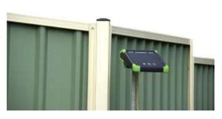
anticlockwise to open the mounting bolt. 4/ Push the Energiser onto the post. Jiggle until you hear the bolt click into the hole. 5/ Rotate the key clockwise to lock. 6/ Make sure the Energiser can't come off. Remove the key. 7/ Put the rubber sealing plug back into the keyhole as an insect & weather seal.
