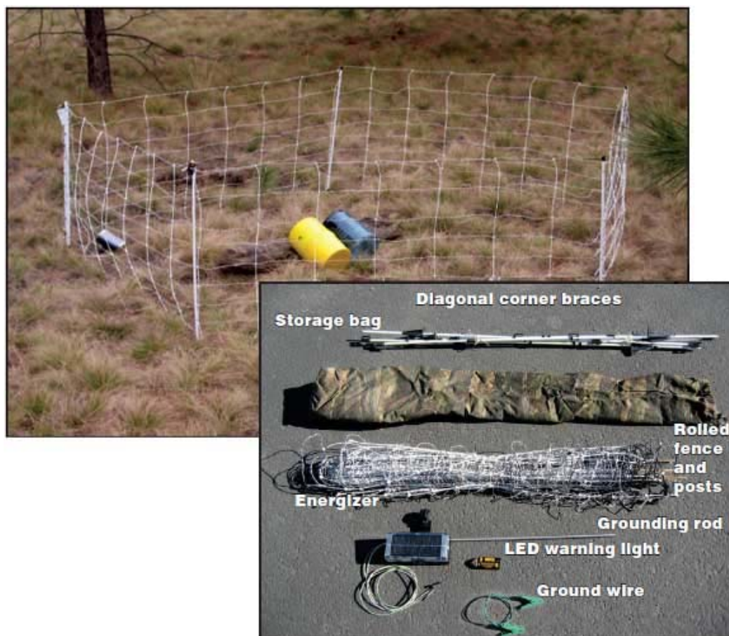
Figure 1—This portable electric mesh fence system is a potential alternative for storing food, garbage, and other attractants in bear country.
