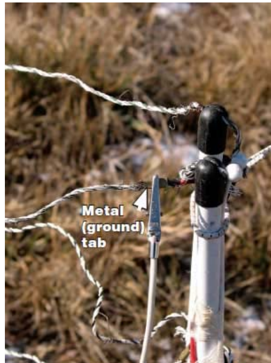
Figure 10—Clip the leads from the energizer to the hot wire (shown) and ground wires of the fence.
